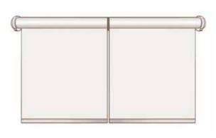
$Minimum\ width\ of\ electric\ drive\ Rollo\ roll-up\ blinds\ with\ 1.1\ Nm\ battery\ (<\pm200\ cm\ x\ 200\ cm/Acmeda):\ 62\ cm\ x\ 200\ cm/Acmeda)$ Minimum width of electric drive Rollo roll-up blinds with 2 Nm battery (> ± 200 cm x 200 cm/Acmeda & Somfy): 75 cm. Minimum width of 230 V electric drive Rollo roll-up blinds (Somfy): 60 cm
