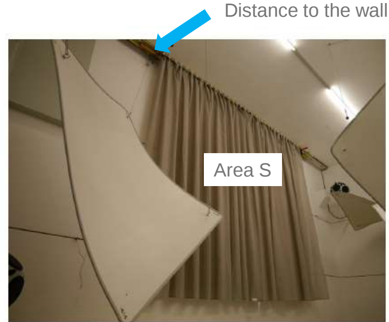
Figure B.2. Folded arrangement, test object mounted in the reverberation room.
